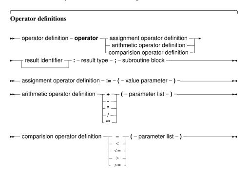
The parameter list for a comparison operator or an arithmetic operator must always contain 2 parameters, with the exception of the unary minus, where only 1 parameters is needed. The result type of the comparison operator must be Boolean.
