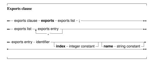
Under Win32, an index clause can be added to an exports entry. An index entry must be a positive number larger or equal than 1, and less than MaxInt.
