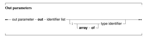
The purpose of an out parameter is to pass values back to the calling routine: the variable is passed by reference. The initial value of the parameter on function entry is discarded, and should not be used.
