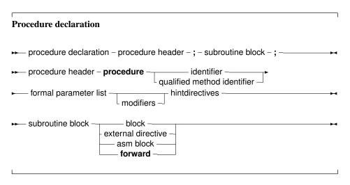
See section 14.4, page 155 for the list of parameters. A procedure declaration that is followed by a block implements the action of the procedure in that block. The following is a valid procedure:
