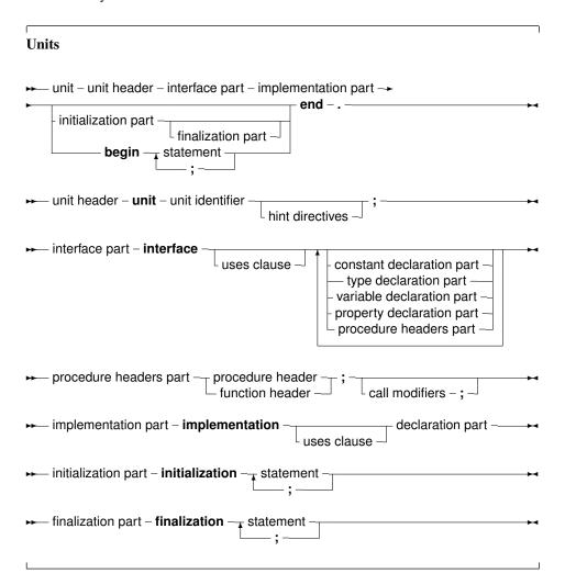
As can be seen from the syntax diagram, a unit always consists of a interface and an implementation part. Optionally, there is an initialization block and a finalization block, containing code that will be executed when the program is started, and when the program stops, respectively.
