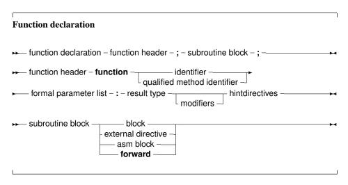
The result type of a function can be any previously declared type. contrary to Turbo Pascal, where only simple types could be returned.
