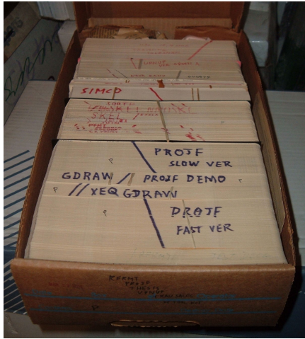
Data and instructions were once stored on external punched cards, which were kept in order and arranged in program decks.
